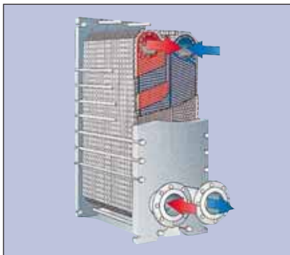
Fig. 1 The all-welded plate heat exchanger consists of a plate pack of herringbone patterned metal plates with portholes for passage of the two fluids. The heat transfer takes place through the thin plates in stainless steel, titanium or SMO and it is a highly efficient heat exchange technique.
